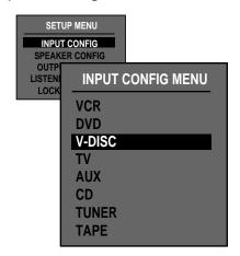
The MC-1 has eight inputs, each of which can be associated with any of the eight video and eight digital audio inputs. Selecting Input Configuration from the Setup menu displays a sub-menu which lists these inputs and allows you to select them individually for adjustment. Each input has an identical parameter sub-menu. V-DISC is shown below as an example.
